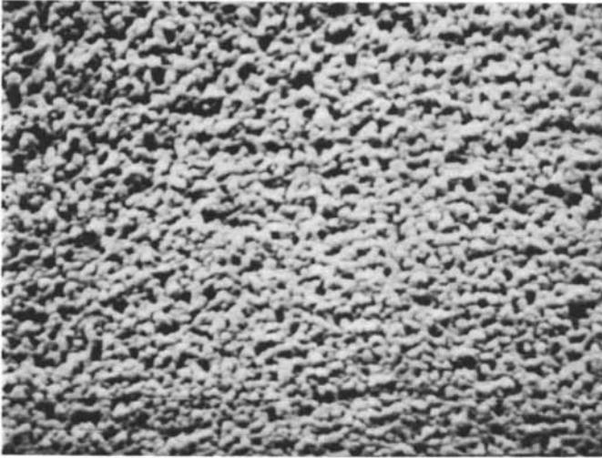
Figure 7a. SEM picture of the dense skin of an asymmetric capillary membrane with entrapped cells. Reproduced with permission from Ref. 14.
